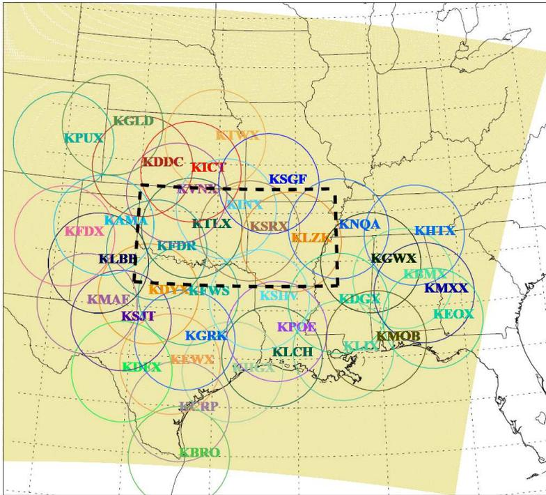
FIG. 3. Model domain measuring 2000 km  $\times$  2000 km (gold) and the 37 NEXRAD radar stations that are used for deriving a 4 km  $\times$  4 km 10 min precipitation mosaic. The four-letter identification code indicates the location and the circles the 230 km radius of individual stations. The simulation is initialized using MERRA vertical profiles averaged inside the dashed black box.
